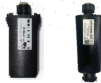
Ai-Dongle can monitor up to 10pcs devices. Wi-Fi-Stick can monitor up to 5 pcs devices.
